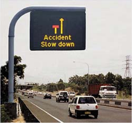
Picture 3 – Example of Variable Message Sign
